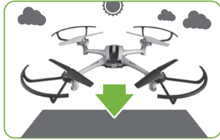
Place the drone on level surface with a clear view of the sky.
