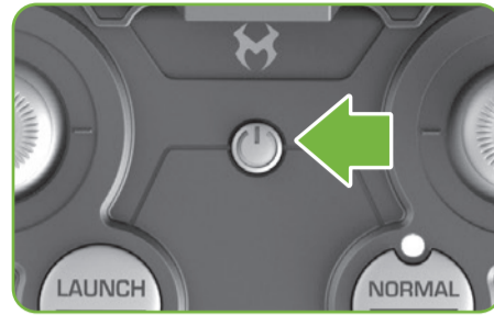
Turn on controller.
