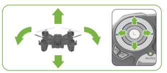
Move **LEFT (Throttle)** thumbstick up or down to make drone fly higher or lower and left or right to rotate.
