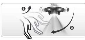
Hold the Aura drone upright in the palm of your hand. Give the drone a slight toss upwards then quickly drop your hand downward. The Aura drone will automatically turn on and hover.
