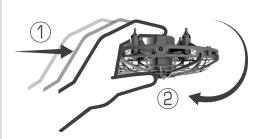
Quickly grab drone and flip upside down to stop. If out of reach, blast drone to make it fall or wait until battery power is depleted. Drone will auto-land itself.
