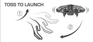
Turn drone on and hold it upright in front of you in the palm of your hand. Keep drone level and give it a slight toss upward, then drop your hand quickly downward. Drone will automatically start to fly. Toss drone high to hover high, toss drone low to hover low.
