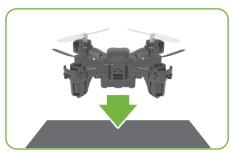
Place the drone on level surface for calibration.
