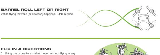
Bring the drone to a mid-air hover without flying in any direction. Remove finger from the RIGHT thumbstick.
