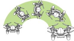
AUTO mode is best for new pilots. Begin by pressing the LAUNCH button for takeoff. The drone will hold its altitude, and gradually fly up or down when you press up or down on the left thumbstick.
