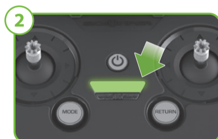
2 When enough satellites are locked on, the GPS MODE will illuminate a solid GREEN. The frame is now ready to fly in GPS mode.
