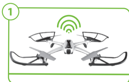
1 The frame will start to acquire GPS satellites. During this time, the GPS MODE LED will blink.
