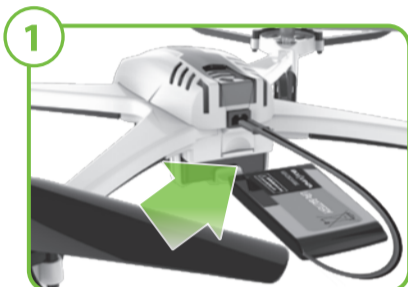
1 Connect Drone LiPo battery.
