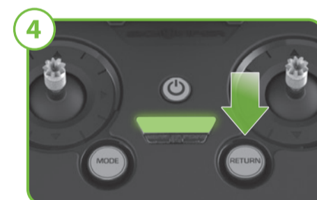
4 When flying in GPS mode, press the RETURN button to RETURN HOME. The frame will fly back to the home location and land. RETURN HOME will ONLY work if GPS MODE is active.
