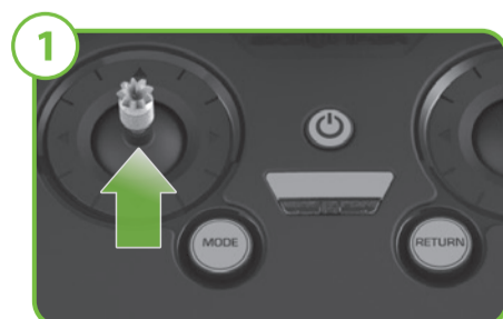
1 Raise the throttle stick to arm the frame. The motors will spin, indicating the frame is armed. Increase throttle to lift off of the ground.
