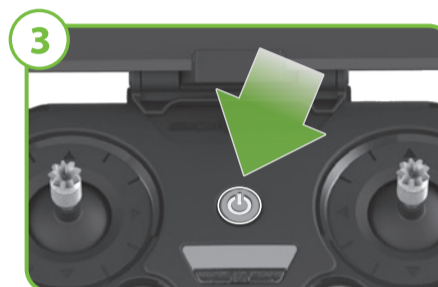
3 Press the power button to turn controller ON.
